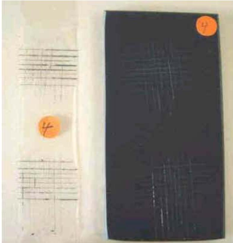
***Figure 5: Test Panel and Adhesive Tape
