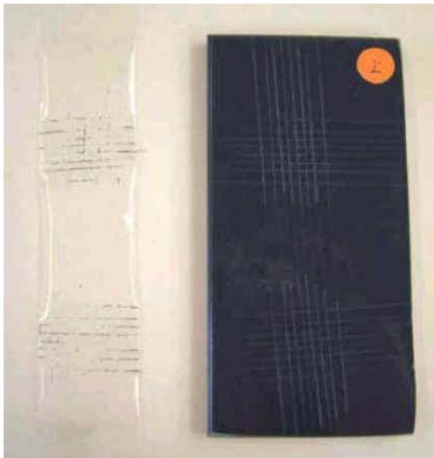
**Figure 4: Test Panels and Adhesion Tapes After the Adhesion Tests**
